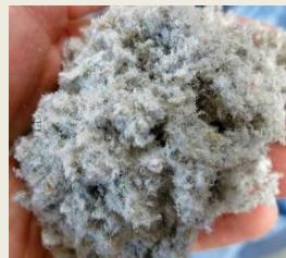
Fig 1: Loose fill cellulose insulation material
